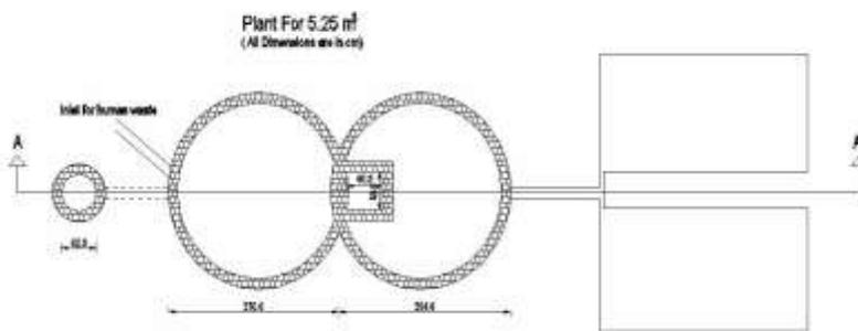
Figure 2: Section of Biogas plant model of a poultry farm
